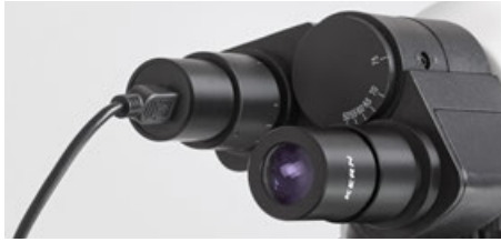
Eyepiece camera fixed into the tube
