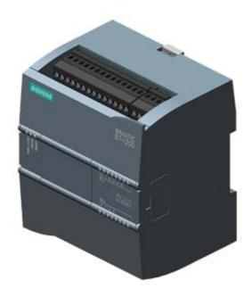
SIMATIC S7-1200, CPU 1211C, COMPACT CPU, AC/DC/RELAY, ONBOARD I/O: 6 DI 24V DC; 4 DO RELAY 2A; 2 AI 0 - 10V DC,
