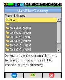
The working directory must be located on the micro SD card, which must be present in the device.
