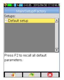
The default setup is one of the predefined configurations proposed in the Main/Setup/Factory menu.
