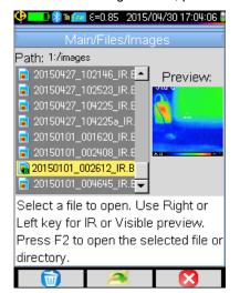
The file manager lists only infrared images generated by the camera bearing a name in the form
