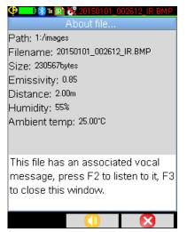
A vocal message is played back using the Bluetooth headset, which must be connected to the camera (see § 6.2.2. How to connect a headset).
