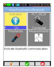
To use this function, you must first activate it from the Main/Parameters/Bluetooth menu by setting the Activation item to "On" (validate the item with F2 , to allow entry, use Up/Down to change the value, and F2 to validate the
