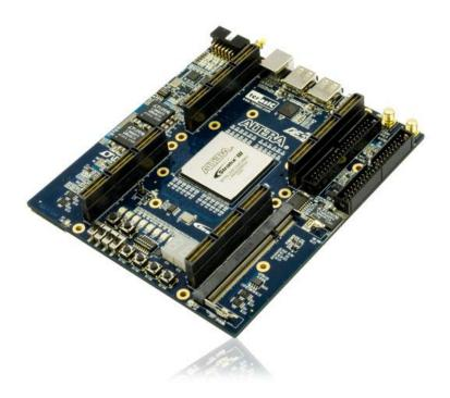
The Altera DE3 ASIC prototyping development board allows researchers and engineers to access the high density and high performance FPGA - the Altera Stratix III. Starting with the Stratix III 3SL150 (142K logic elements), the DE3 is the perfect platform for creating your cutting edge design in programmable logic. The DE3-150 board can be stacked up to create a programmable fabric that is unequaled by any other board system in the world.
