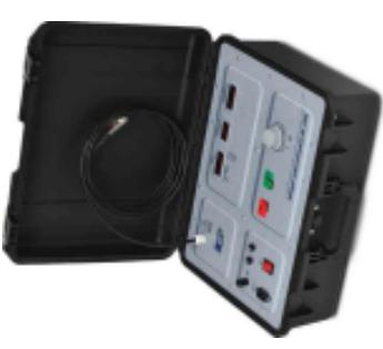
An insulation testing unit AI-2500 with a maximum output voltage of 2500 V AC is intended for insulation testing under AC sine voltage which can be adjusted from 0 to 2500 V (50 Hz). The device can be used in power and electrical engineering industries. Due to increased output current AI-2500 can be used for an AC voltage testing of the winding insulation of large electrical machines and electrical tools.
