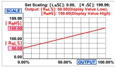
The range between [RaHS] and [RaLS] should be over 20% of span at least; otherwise, it will be got less resolution of analogue output.
