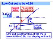
If set the negative value (X2) here to display "X2" which it expressed to be low-cut the PV that it's under the X2 setting value;
