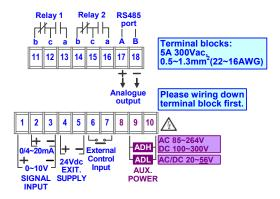
Please check the voltage of power supplied first, and then connect to the specified terminals. It is recommended that power supplied to the meter be protected by a fuse or circuit breaker.
