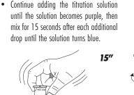
Read off the milliliters of titration solution from the syringe scale and multiply by 300 to obtain ma/L (ppm) CaCO<sub>a</sub>.
