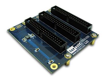
The THDB-H2G (HSMC to GPIO Daughter Board) board is designed to fan out the High Speed Mezzanine connector (HSMC) I/Os to three 40-pin expansion prototype connectors, which are compatible with Altera DE2/DE1/DE0 expansion headers. Users can connect up to three Altera DE2/DE1/DE0 boards (or associated daughter cards) onto a HSMC-interfaced host board via the THDB-H2G board.
