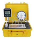
① Connect gauge under test and HS602 on the pressure comparator.
