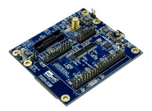
SUM (HSMC to Santa Cruz / USB / Mictor Daughter Board) is an adapter board to convert High Speed Mezzanine Connector (HSMC) interface to Santa Cruz (SC), USB, Mictor, and SD Card interface. It allows users to use these interface on a host board with a HSMC connector.
