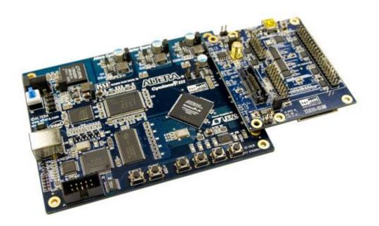
The SUM connects with Altera Cyclone III FPGA Development Board
