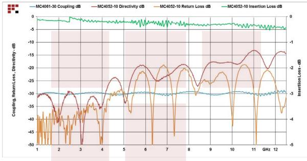
N Directional Coupler 30 dB Coupled Port From 1 GHz to 12.4 GHz Rated To 600 Watts from Fairview Microwave is in-stock and available to ship same-day. All of our RF/microwave products are available off-the-shelf from our ISO 9001:2008 certified facilities in Allen, Texas. Fairview Microwave is RF on-demand.
