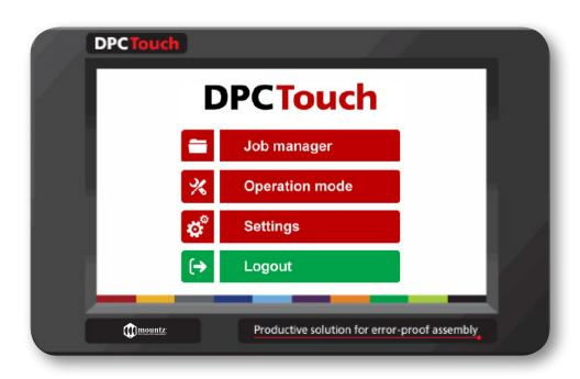
Error proofing and process control to ensure that the torque assembly is completed in sequence and with the correct torque
