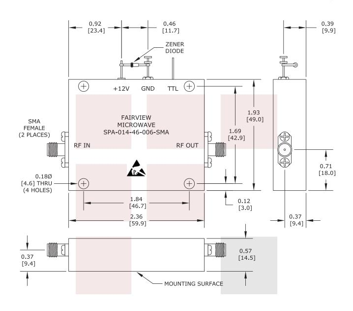
HEAT SINK REQUIRED FOR PROPER OPERATION, UNIT IS COOLED BY CONDUCTING TO HEAT SINK.
