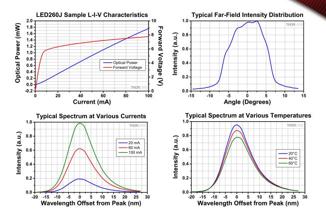
**Note**: The first three graphs show measurements that were made at a case temperature of 25 °C. The last graph shows measurements of the spectrum of an LED held at various temperatures when driven at 100 mA. The far field intensity distribution was taken 25 mm from the LED.
