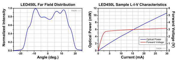
These measurements were taken at a case temperature of 25  $^{\circ}$ C. The output spectrum and radiation distribution were measured with an operating current of 20 mA.
