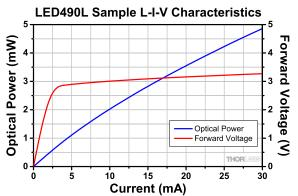
These measurements were taken at a case temperature of 25 °C. The output spectrum and radiation distribution were measured with an operating current of 20 mA.
