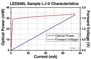
These measurements were taken at a case temperature of 25 °C. The output spectrum and radiation distribution were measured with an operating current of 50 mA.
