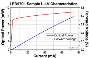
These measurements were taken at a case temperature of 25 °C. The output spectrum and radiation distribution were measured with an operating current of 50 mA.
