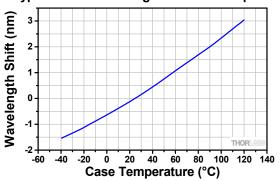
Typical Peak Wavelength Shift vs. Temperature Typical Peak Wavelength Shift vs. Forward Current
