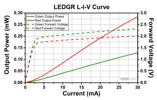
These measurements were taken at a case temperature of 25 °C. The output spectrum was measured with an operating current of 20 mA.
