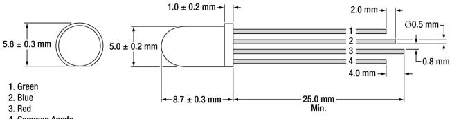
4. Common Anode (Aligns to Flat on LED Housing)
