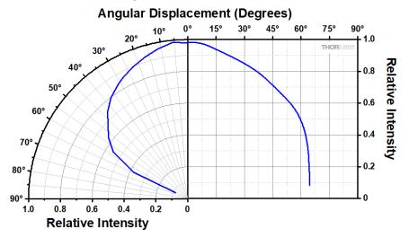
Forward Current and Spatial Radiation Distribution Data Refer to the Bare LED. Spectrum Data was Measured at 25  $\,^\circ C$  with a 440 mA Driving Current.
