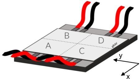
Figure 1: Thermal Position Detector Schematic
