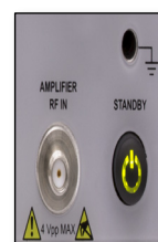
Figure 8 Indicator Glows Green When Instrument Is Fully Enabled
