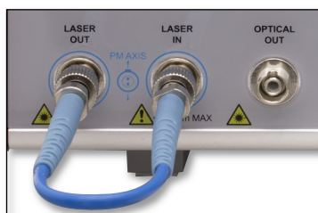
Figure 6 PM Loopback Fiber Cable Installed
