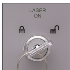
Figure 7 Interlock Key Switch
