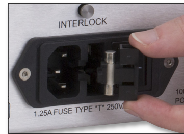
Figure 51 Removing the Fuse Holder Slide
