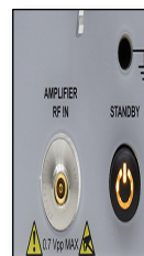
Figure 5 Indicator Glows Amber When Instrument Is in Standby
