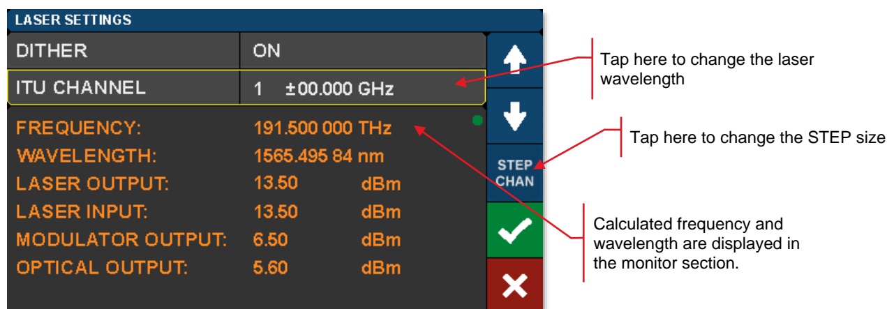
Figure 39 Changing the ITU Channel Number
