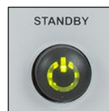
Figure 11 Indicator Glows Green when Converter is Fully Enabled
