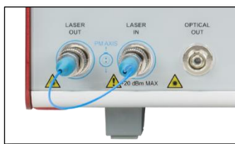
Figure 9 PM Loopback Fiber Cable Installed (Not Available for MX40G-850)
