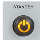
Figure 8 Indicator Glows Amber when Converter is In Standby
