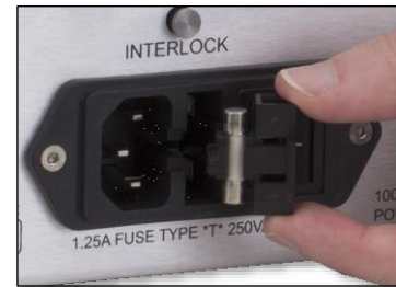
Figure 57 Removing the Fuse Holder Slide
