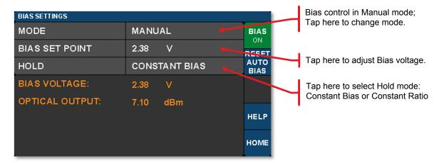
Constant Bias is the most basic mode of operation and will apply a user selected DC voltage to the MZM. This can be useful for performing brief measurements that only take a few minutes. During longer duration experiments, the MZM is more likely to drift.
