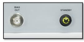
Turn on the MBX by pressing the amber standby button on the front panel until it turns green (about 1 sec) to indicate the unit is fully on. The touchscreen display will come up with a boot screen for about 5 seconds and then go to the home page. The unit will initialize in the factory default state with all functions OFF.
