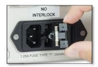
5. Investigate the fuse. This can be done with a simple continuity check. If in doubt, replace the fuse. A spare fuse is stored in the fuse holder. Additional replacement fuses can be purchased from Thorlabs. Always use fuses of the same type as the original.
