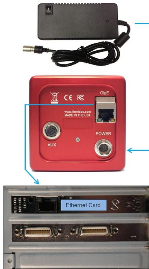
**Figure 3** Diagram of Connectors on GigE configuration
