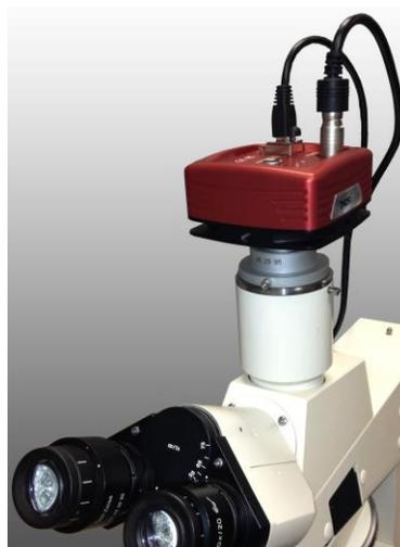
**Figure 7** Camera Shown on Microscope Using C-Mount Adapter
