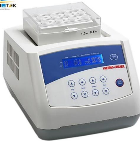
Designed for simultaneous heating and cooling and mixing of small samples, the MSC-100 are supplied with interchangeable blocks for micro tubes. Mixing and heating and cooling modes can be used both simultaneously and independently, i.e. the device can work as a shaker and as a thermostat. The main body of the Mixing Block can be used with different kinds of blocks.
