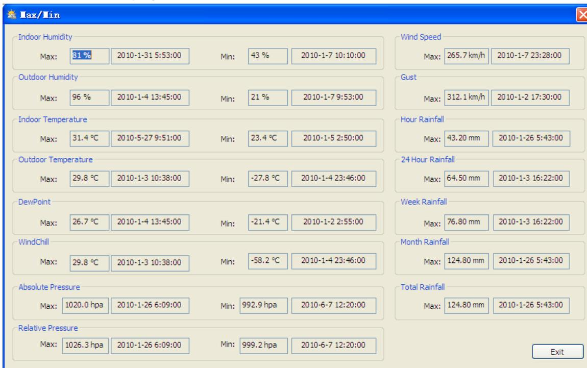
This section is used to display the recorded min and max value values with a time stamp. Min/Max reset can only be carried out on the base station.
