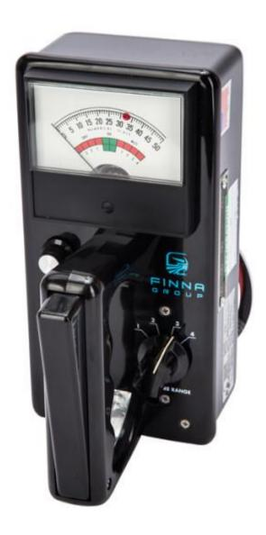
The Model T8 uses the Radio Frequency Capacitance Method to measure the moisture content of products. It operates from a single rechargeable NI-Cad battery. It gives the operator average moisture content down to a penetration of 1/8 to 1/4 of an inch. The electrode has three concentric rings that cover an area 3 inches in diameter. Complete with Rechargeable Battery, Carrying Case and Operating Instructions Book.
