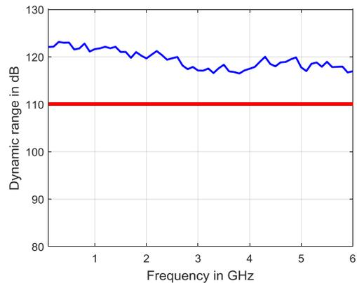
Dynamic range in dB versus frequency for the R&S<sup>®</sup>ZNLE.
