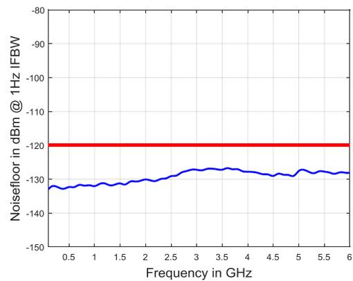
Noise Level in dBm(1 Hz) versus frequency for the R&S<sup>®</sup> ZNLE.
