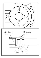
If it is not securely attached, the socket or bit may detach and fly off. Do not attach the socket or bit when the tool is idling.
