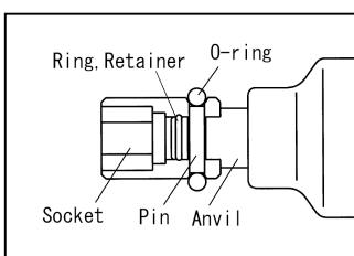
If it is not securely attached, the socket or bit may detach and fly off.
