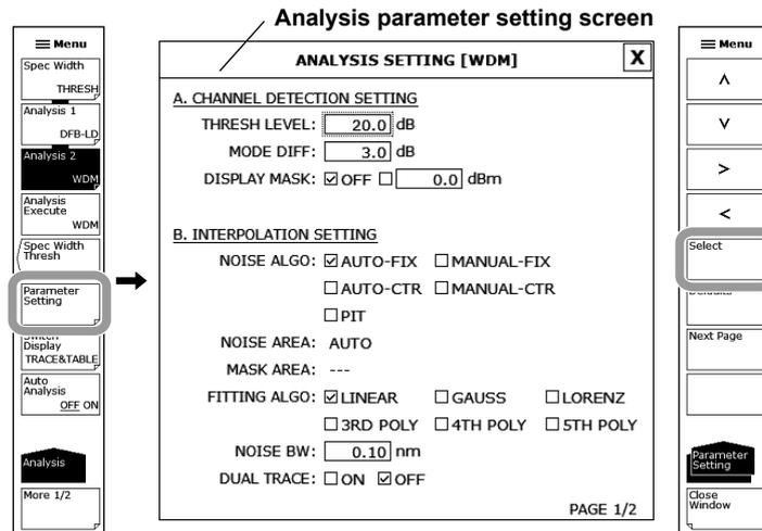
8. Tap **X** to close the WDM parameter setting screen. You can also tap **Close Window** on the function menu. The function menu returns to the previous level.
