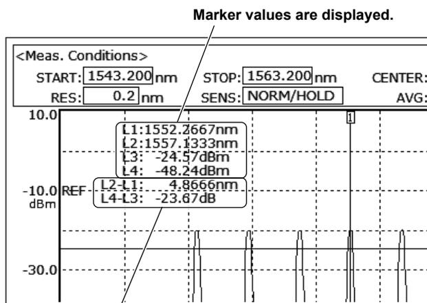
Wavelength difference (L2 – L1) and level difference (L4 – L3) are displayed.
