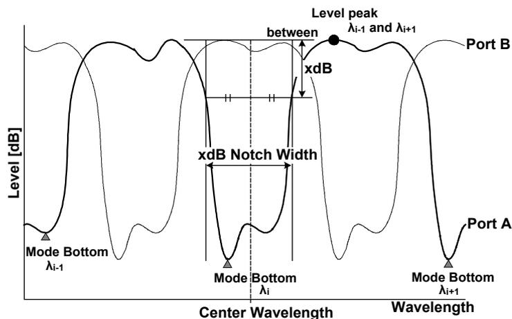
The width (xdB\_Notch\_Width) between the two points, which are below the higher point of either the left peak level or the right peak level of each channel by the parameter THRESH\_LEVEL, and its center wavelength/frequency (Center\_Wavelength) are determined.
