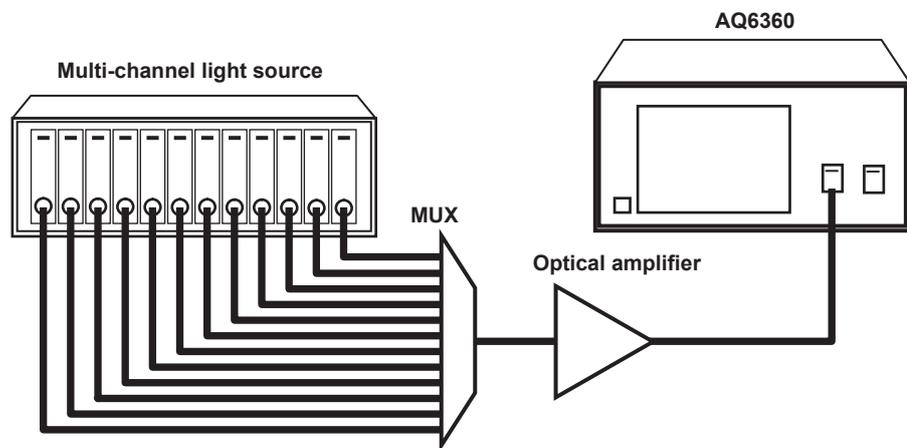
WDM signal light is measured, and the waveform is drawn in the active trace.
