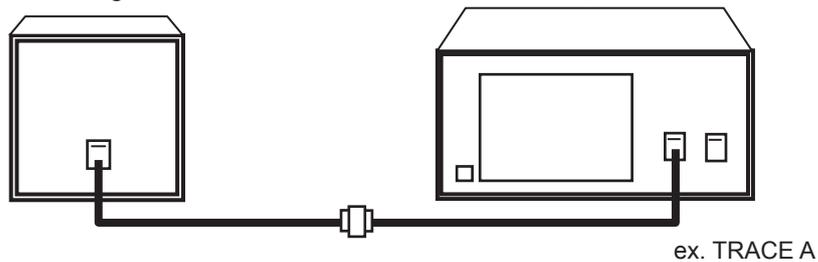
Spectrum measurement after passing through the filter
