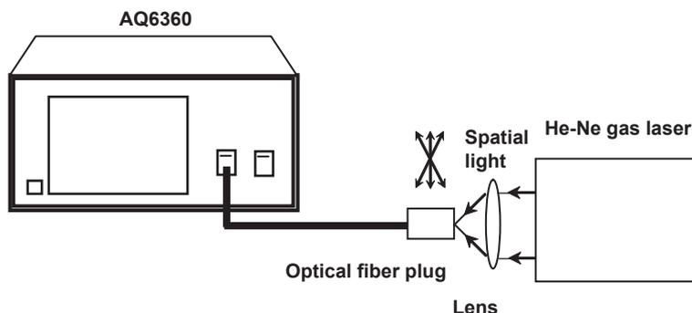
The sweep width is set to 0 nm, the center wavelength is fixed, and the level of a single wavelength of light is measured.
