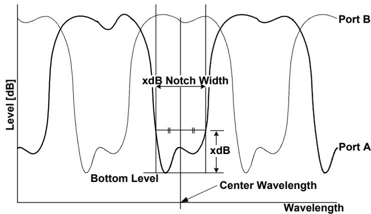
The width (xdB\_Notch\_Width) between the two points, which are above the bottom level of each channel by the parameter THRESH\_LEVEL, and its center wavelength (Center\_Wavelength) are determined.
