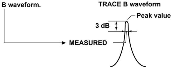
If the RES BW parameter is set to “CAL DATA,” the resolution bandwidth stored in the instrument is used.
