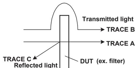
The value of  $k$  is an absorption coefficient which is used in determining the DUT reflectivity and transmission efficiency. Different algorithms are used depending on whether transmission efficiency or reflectivity is estimated, so the  $k$  value also varies accordingly.
