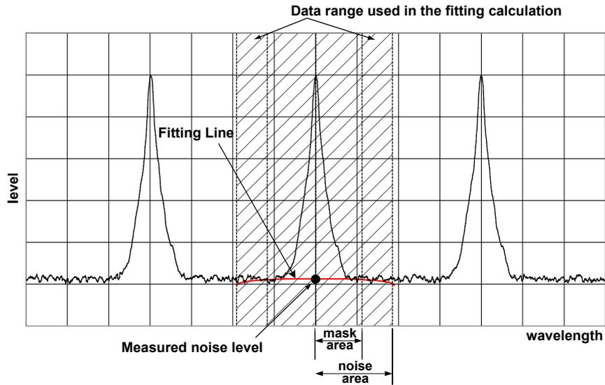
1. Channel detection is performed on the measured waveform data according to the following procedure.
