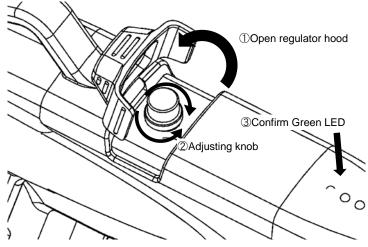
②Rotate knob of regulator to supply appropriate amount of air to motor cartridge. The ring under knob is stopper.
