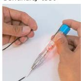
A conductivity check of electrical Continuity check of a wiring circuit Make sure that no power is applied to the circuit before checking continuity.
