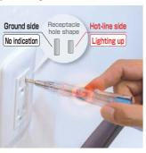
wiring or receptacle and polarity discrimination of AC hot-line and ground sides
