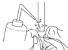
2. **Open the internal solution filler port of the electrode.**
