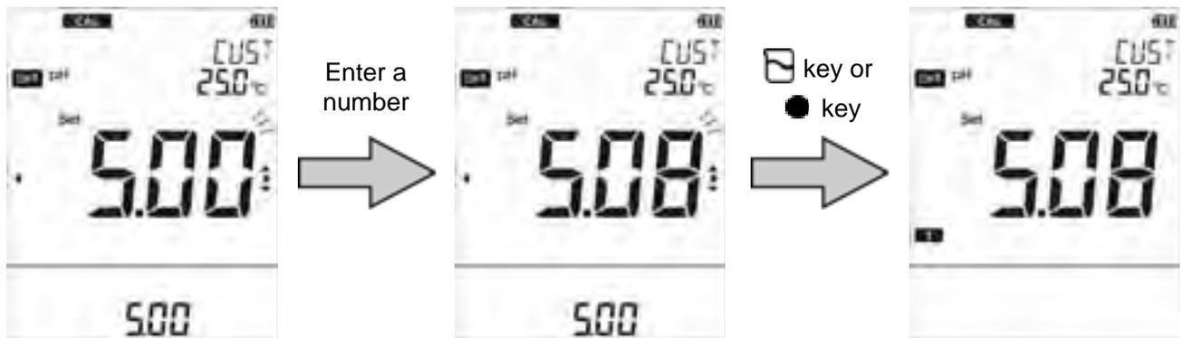
6. Perform the 2nd point calibration. As with the step 1., clean the pH electrode and immerse it in the 2nd standard solution. As with the step 3., immerse at least 3 cm from the tip of the pH electrode.
