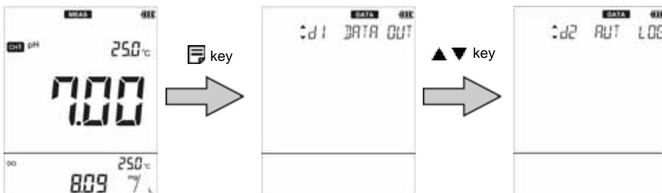
3. Enter the interval of saving in seconds and press the
