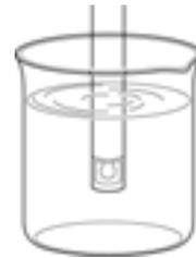
7. Press the
