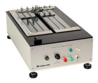
• This tester is used to evaluate the drying characteristics of paint.
