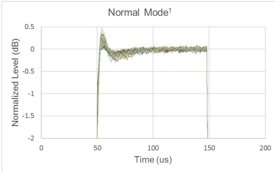
1. Measured with a 500 kHz IF bandwidth, averaging factor of 16 (Average Type = Point). With 100 us pulse width setting. 50 usec/div.
