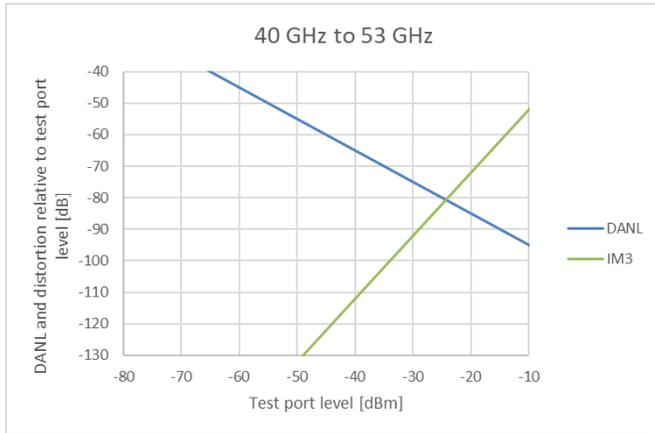
2. With High Attenuation. 2<sup>nd</sup> harmonic distortion applies up to 26.5 GHz.
