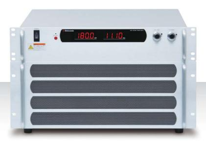
AUH series is high performance HV power supply which can output ultra high voltage of maximum 200kV in the 19-inch rack size. By the safety design without the exposure of the high voltage output part, quantity of outbreak of the corona is held down as compared with the open type power supply.
