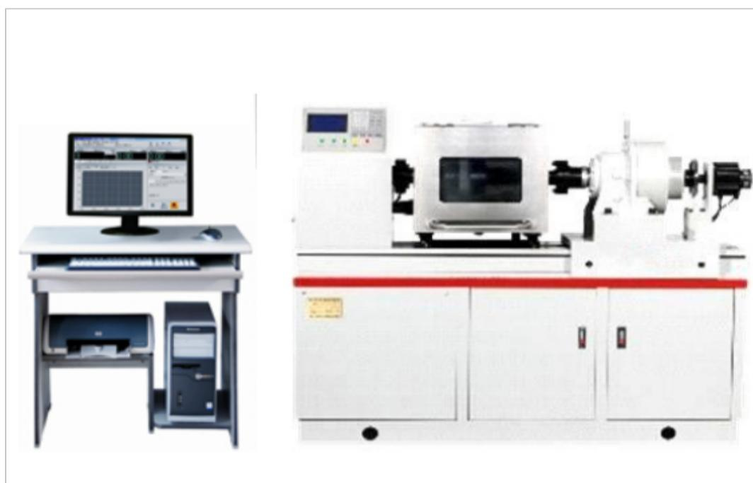
(<http://wenku.baidu.com/s?wd=High and low Temperature Torsion Testing Machine&tn=SE hldp08010 vurs2xrp>)
