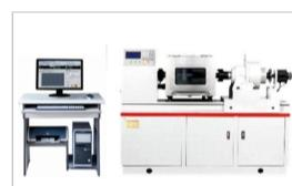
High and low Temperature Torsion Testing Machine
