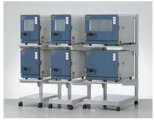
Sample installation of stacking stand (optional)
