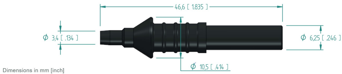
Figure 4 Probe tip adapter dimensions
