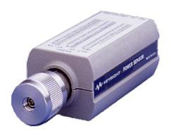
The 8485D diode power sensor measures average power over the frequency range 50 MHz to 26.5 GHz and power range -70 to -20 dBm (50 dB dynamic range).
