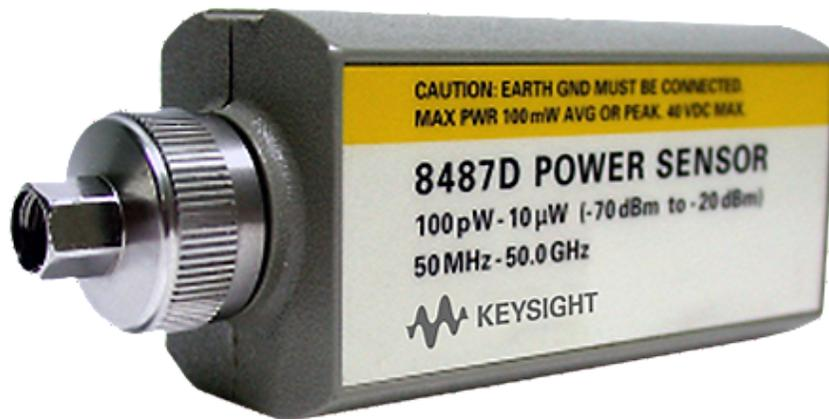
The 8487D diode power sensor measures average power over the frequency range 50 MHz to 50 GHz and power range -70 to -20 dBm (50 dB dynamic range)
